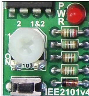
Potentiometer for test Mode & voltage selection button
