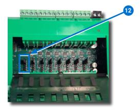
**NOTE:** Each of the eight override slots ships from KMC with a jumper installed on the two pins closest to the output terminal blocks. Only remove a jumper if an override board will be installed.
