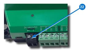
NOTE: Connect only one controller to each 24 VAC, Class-2 transformer with 12-24 AWG copper wire.
