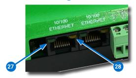
The **Ethernet status LEDs** indicate network connection and communication speed.
