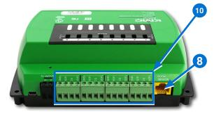
**NOTE:** Auxiliary VAV equipment such as fans, heaters, reheat valves, and discharge air temperature sensors can be connected to the controller.
