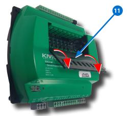
14. Remove the **jumper** 12 from the slot in which the override board will be installed.
