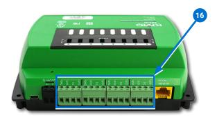
**NOTE:** HPO-6701 triac and HPO-6703/6705 relay board circuits use the Switched Common **SC** terminal—not the Ground Common **GND** terminal.
