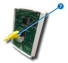
**NOTE:** The Ethernet patch cable should be a maximum of 150 feet (45 meters).
