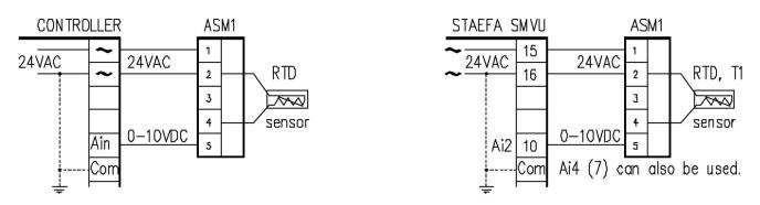
The ASM1/RTD-1K/10V/0-100/S or ASM1/T1/10V/0-100/S interface module is factory set up to receive a 0 to 100°F resistance signal from a RTD or STAEFA's T1 temperature sensor and provide a voltage output inputs. The stand-alone version provides an internal pull-up resistor, while the parallel version has a high input impedance as to not load the existing sensor circuit.
