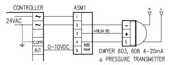
The ASM1/mA3/VDC//P (potted version) is factory configured to provide +18.5VDC power for 3 wire (positive referenced) 4 to 20mA transmitters. The input has an internal 62 Ohm load resistor, referenced to the 18.5VDC supply, as required by DWYER's 603 and 606 transmitters. The load resistor produces a .24 to 1.24V signal that is scaled to the desired output signal.
