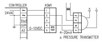
The ASM1/mA/VDC/P (potted version) is factory configured to accept the 4 to 20mA signal from a 4 wire transmitter. The 4 to 20mA signal is fed into a 62 Ohm load resistor, referenced to common, and provides an adjustable voltage output from 0 to 3V to 0 to 10VDC.
