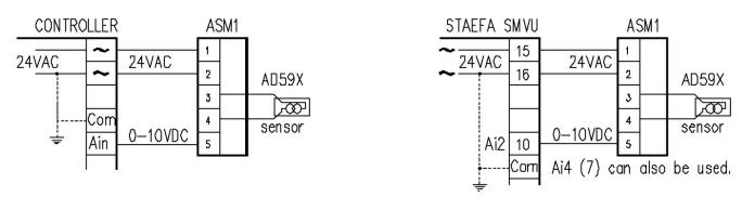
The ASM1/AD59X/10V/0-100/P interface module is factory set up to provide a +15VDC power source for an AD590 or AD592 temperature sensor and receive a 0 to 100°F signal and provide a 0 to 10VDC output. The ASM1 output is scaled for a specific temperature range allowing other sensors to be used with controllers that have a specific sensor type input.
