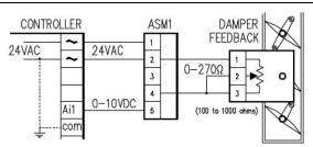
The ASM1/Ohms/10V or VDC interface module can be factory configured for 2 or 3 wire potentiometer (resistance) inputs. A pull-up resistor is connected between the input and the internal voltage regulator to provide one half of a voltage divider circuit while the potentiometer provides the second. This application could be used to provide a manual positioning potentiometer or to read the damper position from a feedback potentiometer and generate an adjustable voltage output.
