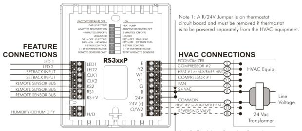
Note 2: Check Heat Pump Installation Instructions for reversing valve connection, either 'O' or 'B'.
