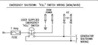
A double pole kill switch wired and installed by the user, stops the generator instantly in emergency situations such as a fuel spill. One switch pole (N.C.) kills power to the GSCM-mini opening all relays. The other switch pole (N.O.) shorts out the magneto for an instant stop.
